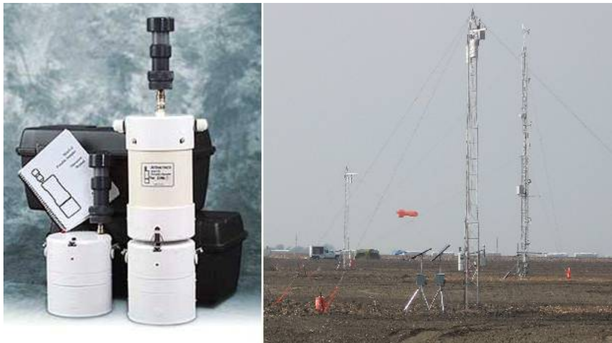
Figure 10. Airmetrics MiniVol Portable Air Sampler, a closeup view and an example of field deployment.
