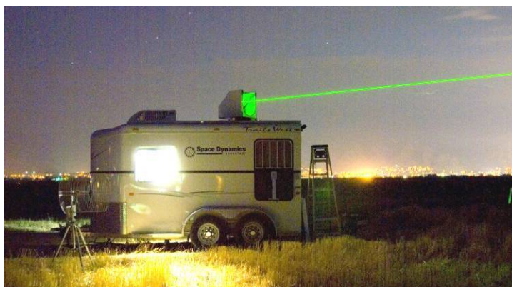
Figure 12. The three wavelength Aglite lidar at dusk, scanning a harvested wheat field.
